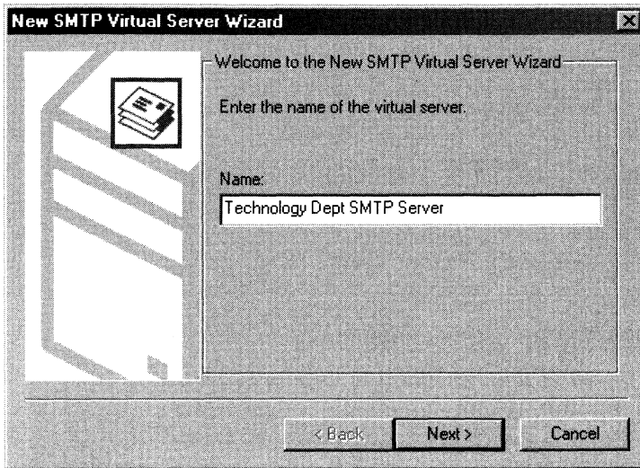
Figure 13-5. Use the New SMTP Virtual Server Wizard to create the additional virtual server
