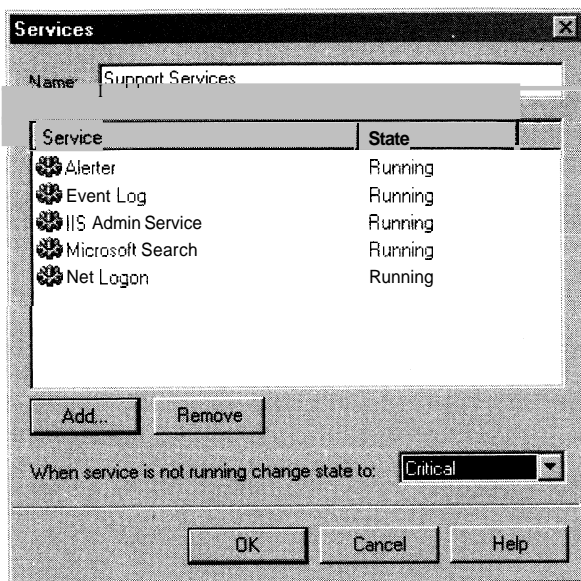
Figure 15-10. In the Services dialog box, type a name for the group of services you want to monitor. Then, after adding the services, set the type of alert as either Warning or Critical.
